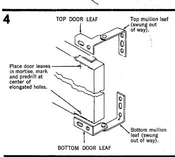
To allow for vertical adjustment and sufficient clearance under the door, the bottom mullion leaf should be mounted at least 1/4" off the floor. If carpet or other special floor coverings are used, additional clearance should be allowed equal to their thickness.
