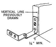
Apply bottom hinge to face of multion using the center of the elongated hole. Be sure to line up with previously drawn vertical line.
